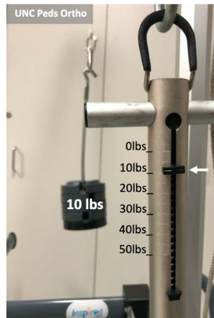
Figure 3. Spring-based HGT system demonstrating 10lbs of hanging weight with corresponding correct reading on the scale (white arrowhead). When the system is applied to a patient with the head/halo in a fixed location, the tension is added by shortening of the rope using a pulley system (simple or block pulleys).
