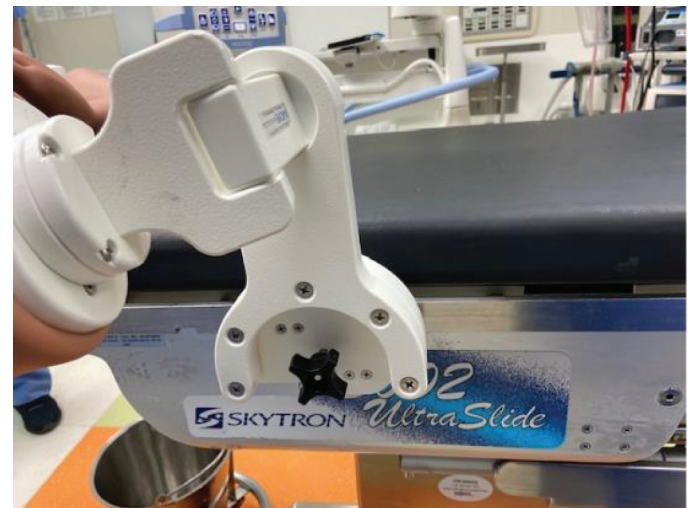
Figure 5. Close up view of the clamp used to attach the simulation model to the OR table. A series of three hinges allow for motion in three planes and mimics motion at the shoulder for a patient who is positioned at the edge of the table with their arm off the table.
