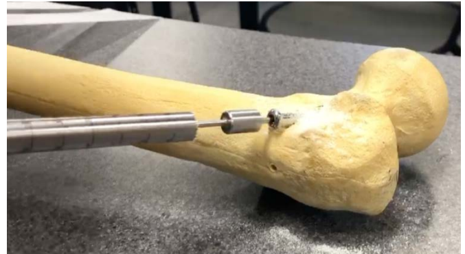
Figure 10. Wire guided assembly ensures coaxial alignment
